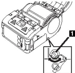
6. Turn the label roll lightly by hand and confirm that it rotates smoothly. Otherwise, paper may not be fed correctly during operation.
